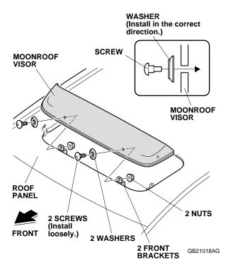
15. Loosely install the moonroof visor to the side brackets with two screws, two washers, and two nuts. Remove the masking tape from the side brackets.
