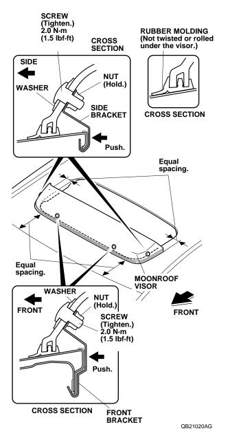
17. Tighten the two screws on the side of the opening first, then tighten the two screws on the front. Apply pressure so that there is no gap between the brackets and the roof panel. Torque the screws to 2.0 N·m (1.5 lbf·ft). 18. Remove the IMPORTANT INFORMATION label and the shop towels.
