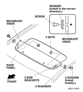
16. Position the moonroof visor with equal spacing in the front and on the sides. Check that the rubber molding is not twisted or rolled under the visor.
